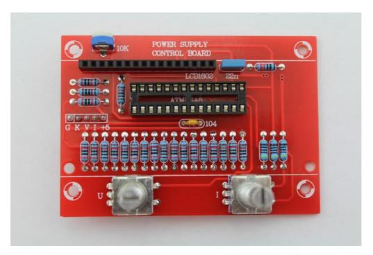
Connect M8 and the LCD which is welded with the insert pin. Be aware of the direction of IC.
